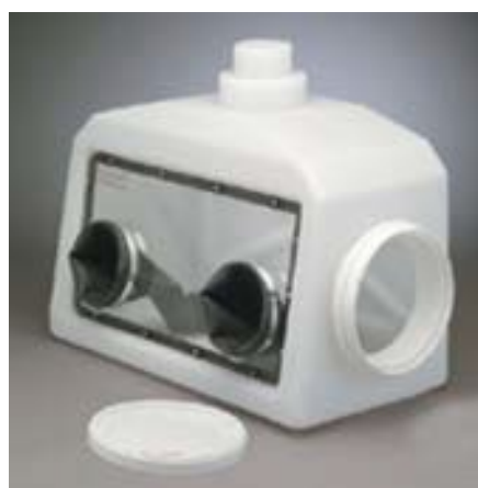
Glove box with venting capability
