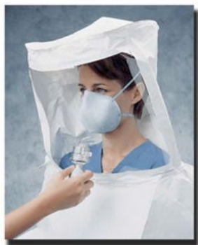
Fit testing an N-95 with Bitrex™
